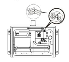
8. Remove end cap from blind plug. Pull wires and earthing through the flexi hose and air branch on motor. Fasten the flexi hose to the cabinet branch. Attach the opposite end of the flexi hose to branch on tap.
